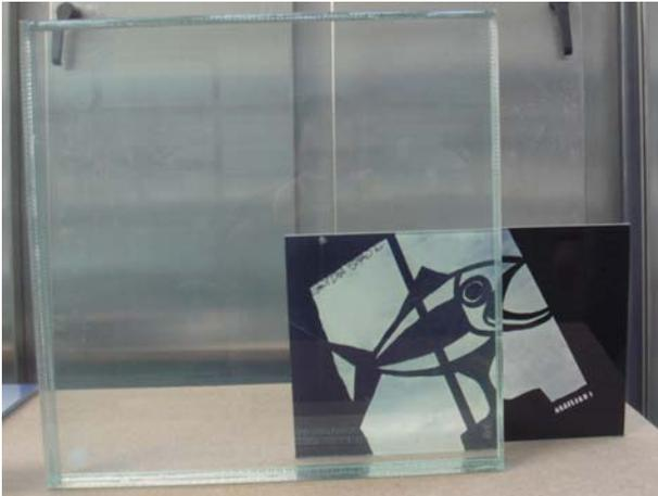
Figure 10: Sample of a heat strengthened laminated pane 500 mm x 500 mm consisting of 6 soda-lime low iron 12 mm thick plies laminated with 1.52 mm thick ionoplast film. Courtesy of Cristec
