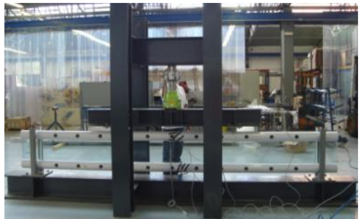
Figure 11: Full-scale four-point bending test set-up
