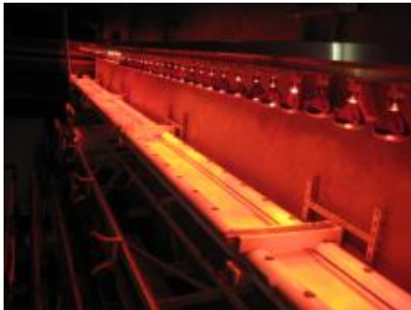
Figure 8: Conditioning of the fin by infrared heating lamps
