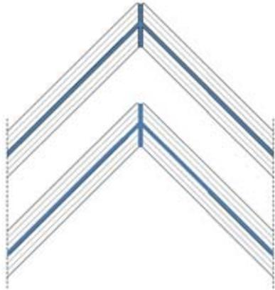
**Figure 1** IGU mitred joint as built section
