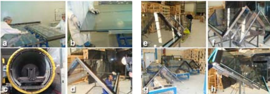
**Figure 6** IGU bespoke production process steps.
