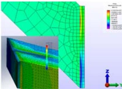
**Figure 5** 2D and 3D mitred joint FEM
