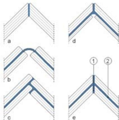
**Figure 3** Several mitred joint concepts including solution finally adopted.
