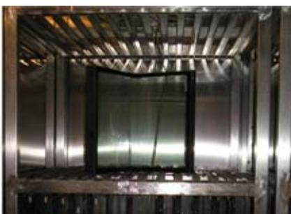
**Figure 8** Sample inside ageing chamber. Courtesy of APPLUS.
