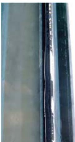
**Figure 7** Delaminations on SGP mock-up's mitred joint.
