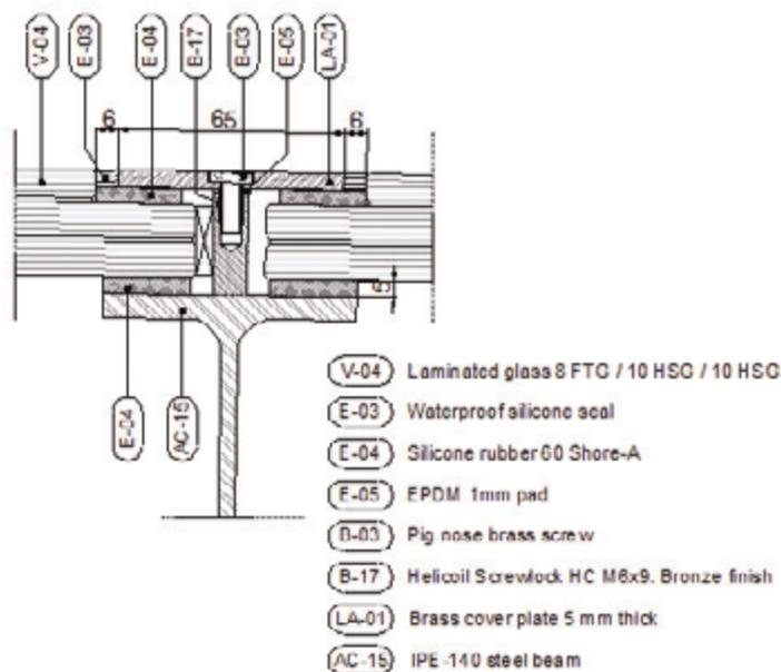
Figure 2. Detail of the glass floor
