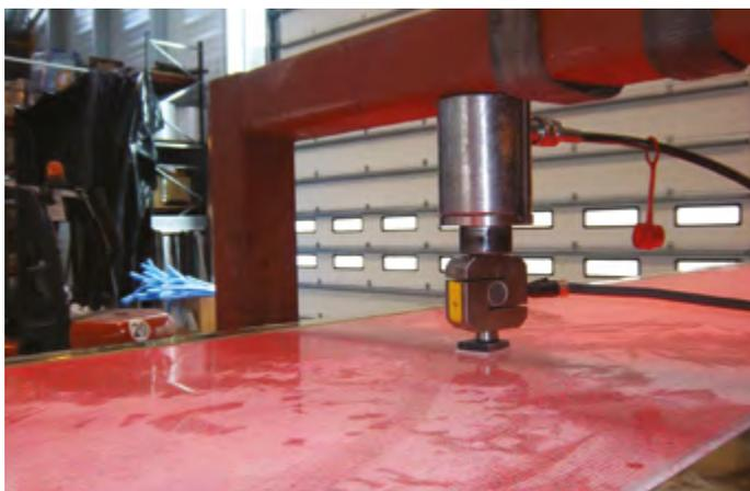
Fig. 4. Point loading test of 2 kN
