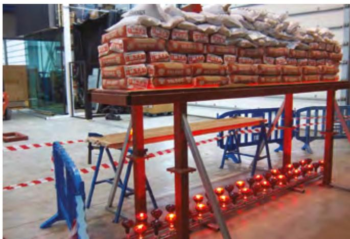
Fig. 5. Load bearing capacity test on the glass panel under ULS (9 kPa)
