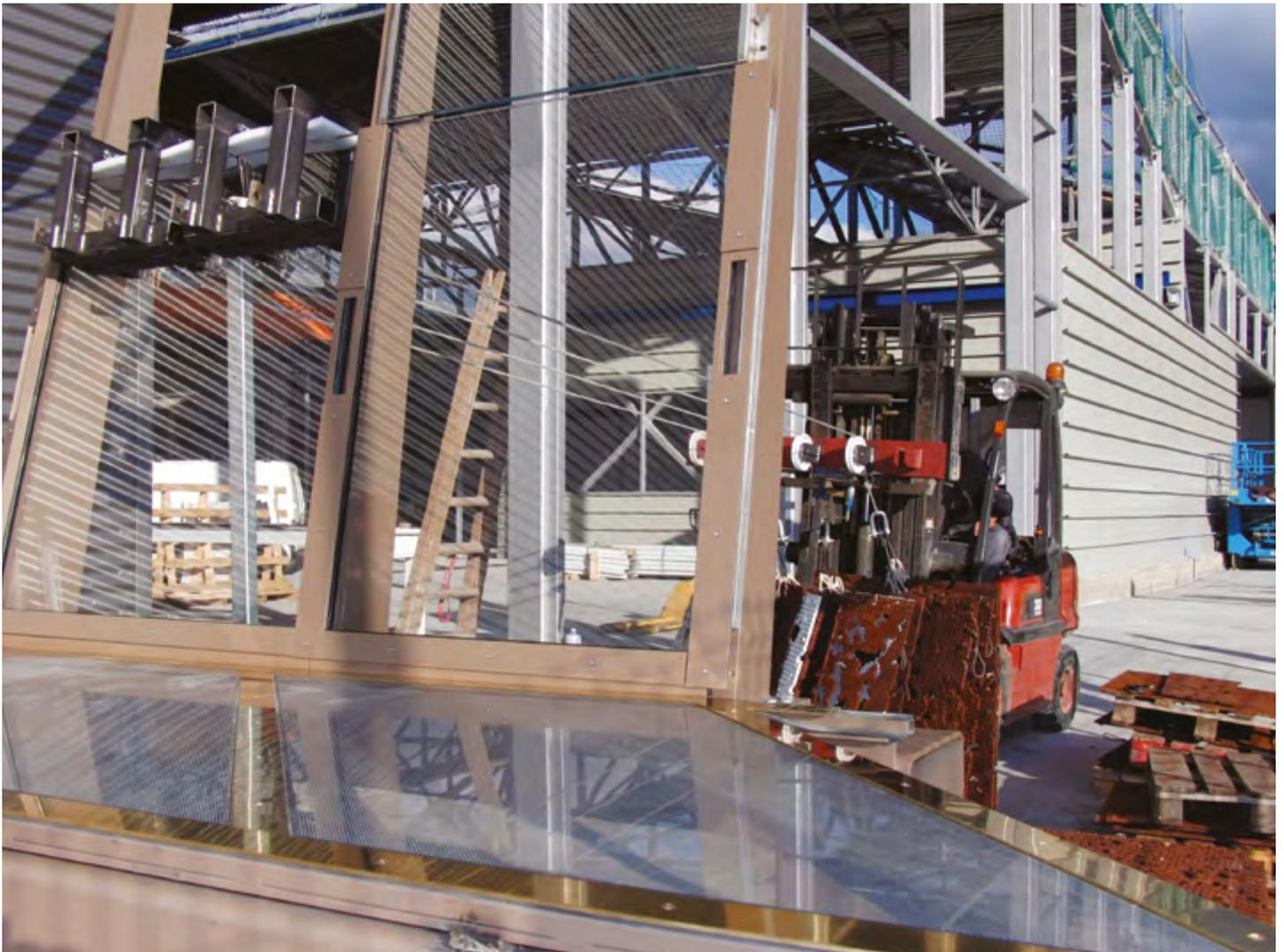
Figure 7. Application of an horizontal factored load of 9 kN/m
