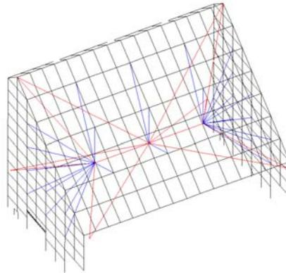
Fig. 2: Steel structure. Tension rods and central shaft in red. Tubular struts in blue.
