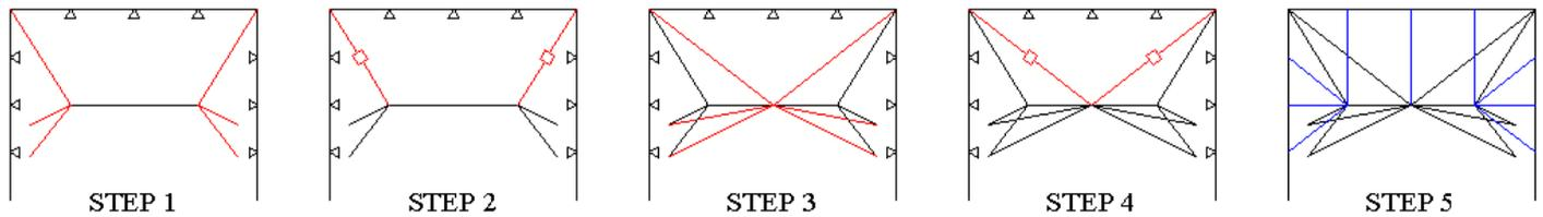
Fig. 6: The prestressing operation
