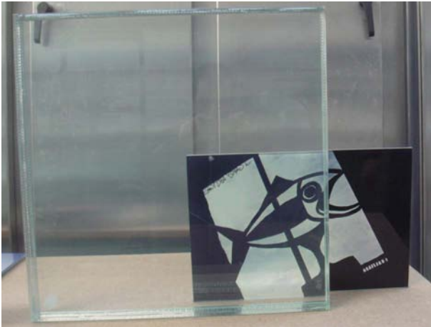
Figure 10: Sample of a heat strengthened laminated pane 500 mm x 500 mm consisting of 6 soda-lime low iron 12 mm thick plies laminated with 1.52 mm thick ionoplast film. Courtesy of Cristec
